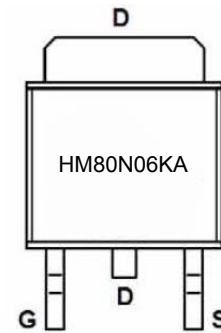
Marking and pin assignment
