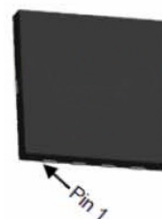
DFN 3.3x3.3 EP top view
